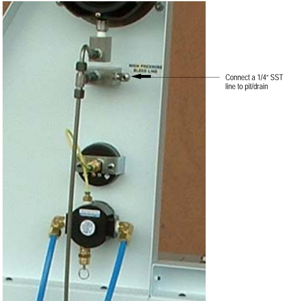
Figure 4-3b.1 Digital GTC Console Plumbing
