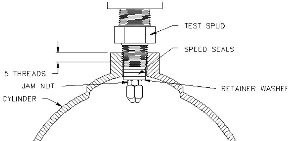
Figure 3 - 1 Hydraclose Seal
