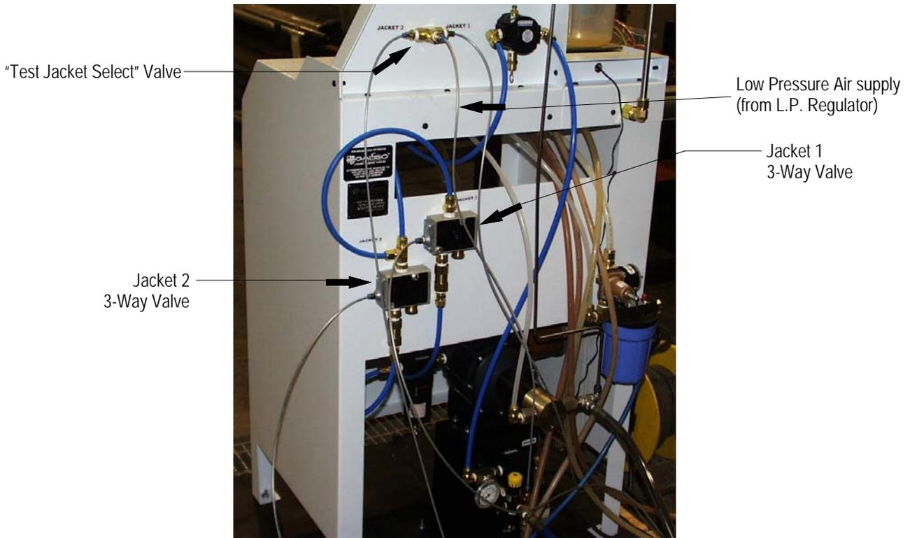
Figure 7-2 Interlock Parts-Rear of Console
