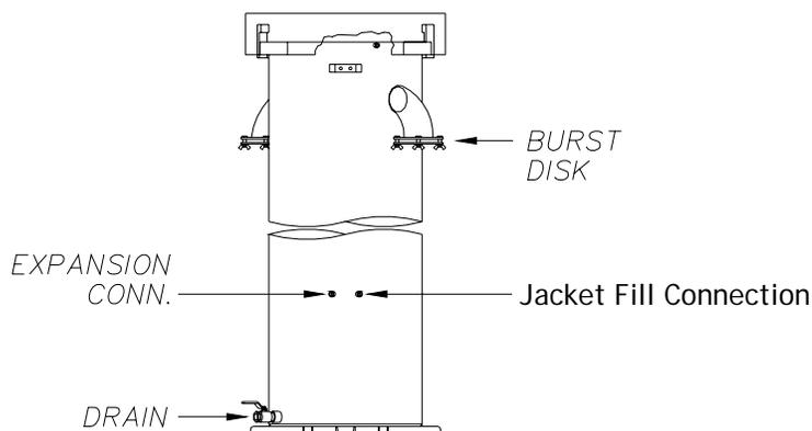
Figure 4 - 4 Hydraclose Test Jacket
