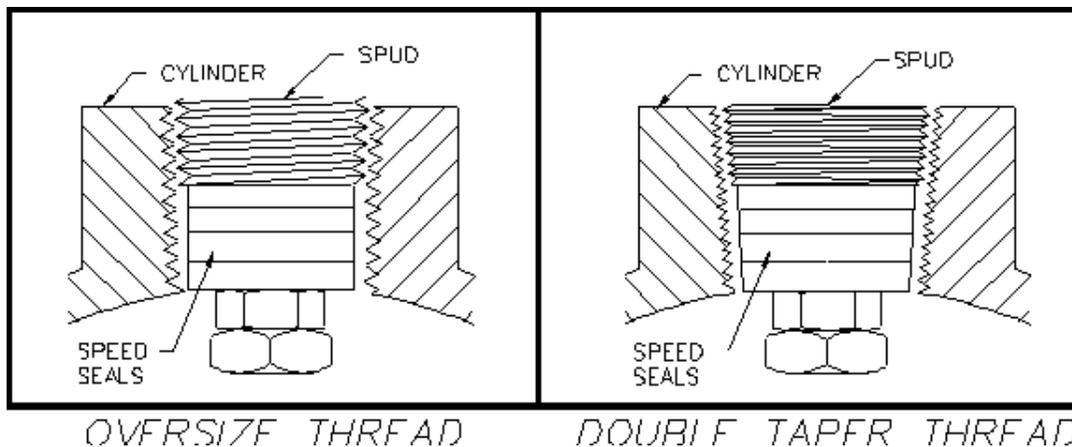
Figure 3 - 2 Cylinder Neck Thread Detail
