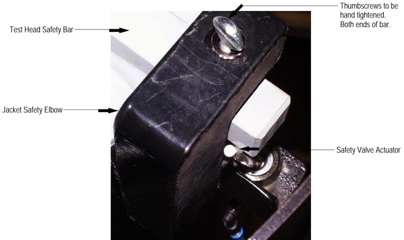
Figure 7-3 Interlock Actuator
