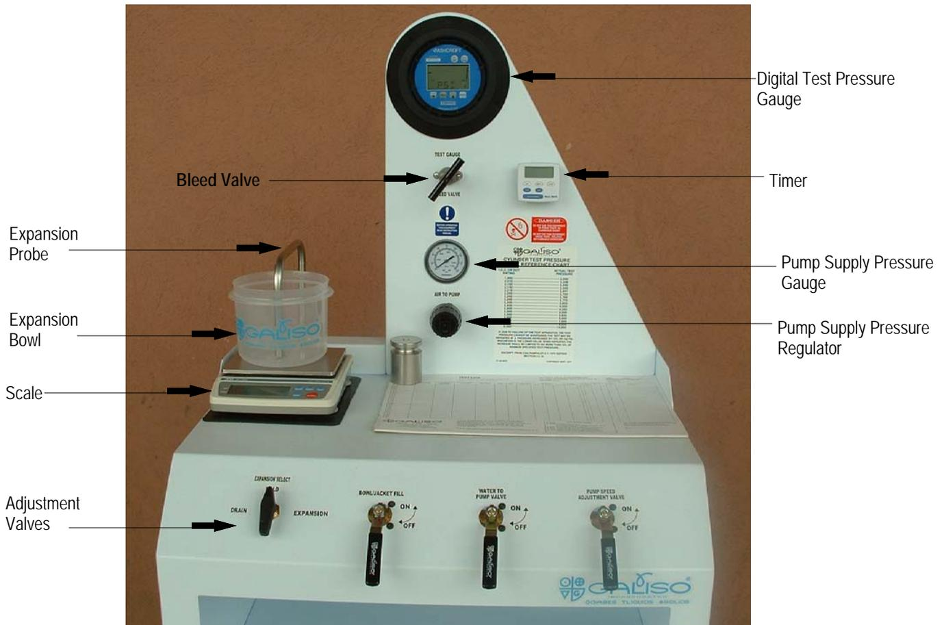
Figure 2- 1 Digital GTC Test Console
