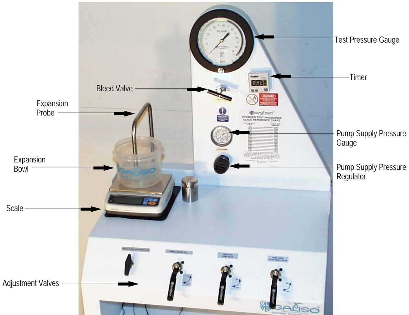
Figure 2- 2 Analog GTC Test Console
